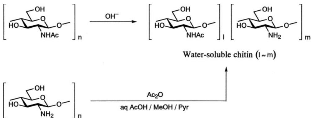
**Figure 6:** Deacetylation of chitin in a hydroxide solution and acetylation of chitosan to create water-soluble chitin (*Kurita, 2001*)
